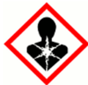
Serious Health Hazard
